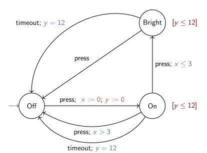
A timed automaton is a finite automaton with one or more real valued clocks. Transitions are annotated with resets and guards and states may be annotated with invariants.
